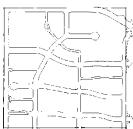
The images at left illustrate three conceptual subdivision layouts. The top image is an example of a poor layout with too few connections and many dead ends. The lower two images show improved street layouts with the required connections and a network of streets. (Diagrams courtesy of Fort Collins, Colorado)
