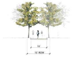
D. Surface Materials: Compact gravel, concrete, asphalt, or other material approved by the Administrator.
